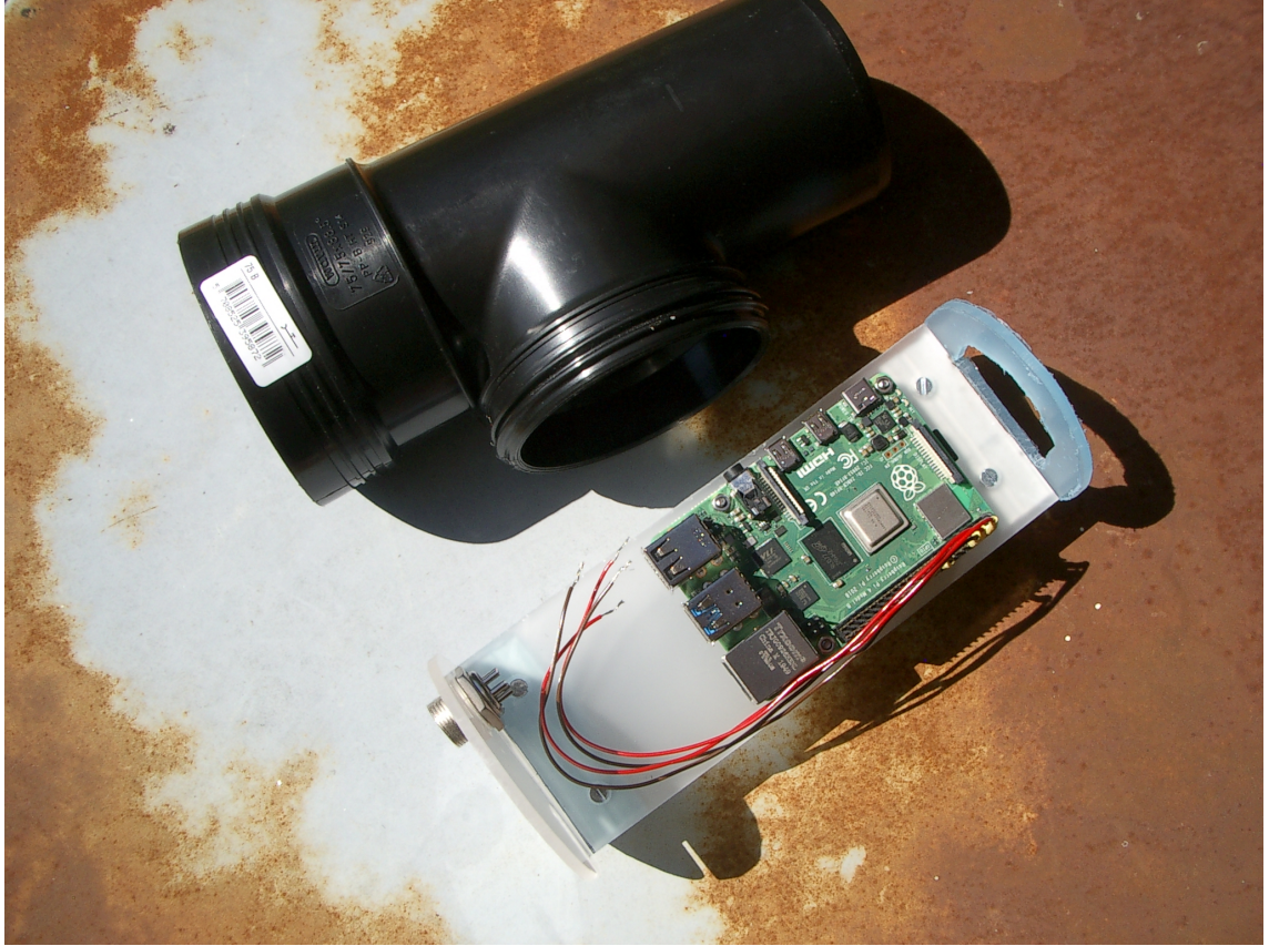
Figure 11: Insert for 3 inch camera housing, with PI 4
