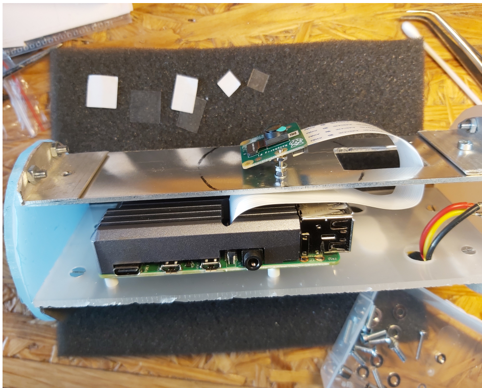
Figure 12: Insert for 3 inch camera housing, nearly complete
