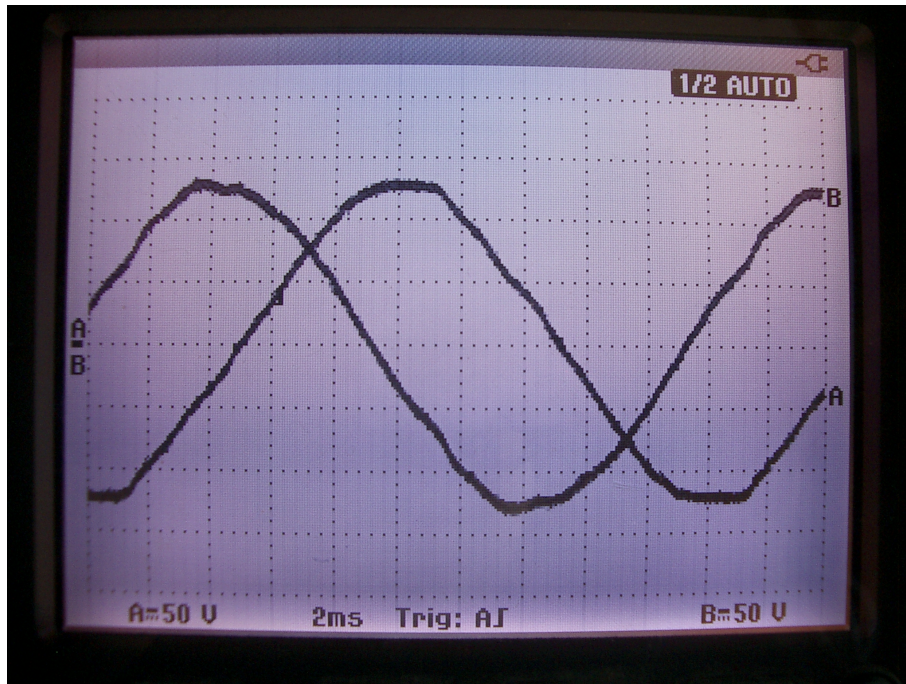
Figure 7: Motor winding voltages on red (ch A) and blue (ch B) wire
