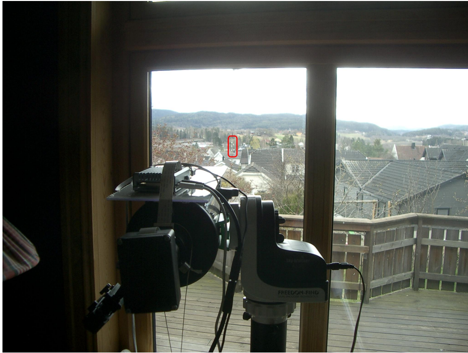
Figure 5: HQ camera mounted on the telescope
